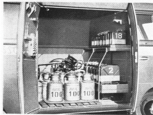
VW Box Van with racks for special oil and lubricant containers for the airport ground service crew.
